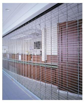
Are open design grilles allowing free circulation of air and full visual access to the area being protected. The curtain is comprised of a series of 5/16" diameter solid aluminum (stainless or galvanized optional) rods of alloy 5056 H32 at 2" on center (1 1/2" optional). Supporting the horizontal rods are vertical chains formed of eyeletted aluminum (stainless optional) spaced at 9" apart. For added security, the chains may be specified to be spaced at 6" or 3" apart.
