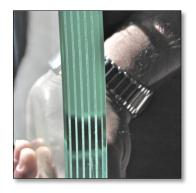
FIRESWISS is a specially fabricated multi-laminate fire-rated glazing material that not only survives a fire to protect against smoke, but also insulates against heat.
