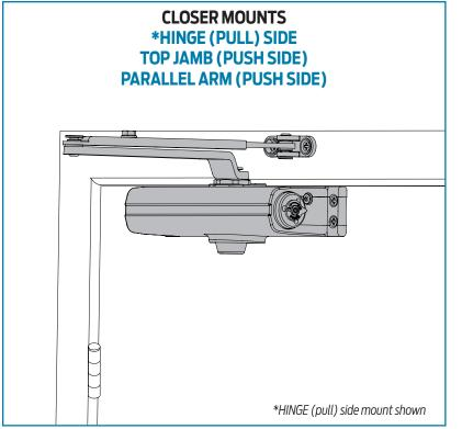
The 1260 is a light to medium duty cast iron closer designed to fit into the most common commercial foot print. The 1260 is adjustable for spring sizes 1-5. The 1260 also features a complete line of regular and extra duty arms, LCN's peel-n-stick installation templates, a convenient spring adjust pointer, and an optional Quick Fix™ bracket kit.
